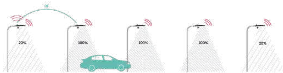
Figure No. 6.3.4.1 : Proposed Smart Street Lightning System
